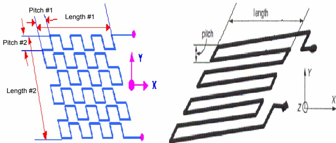
**Figure 1:** Configuration of planar electromagnetic sensors, mesh and meander type
