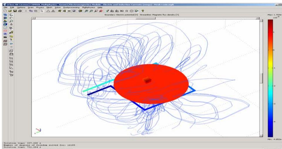
**Figure 12:** Magnetic flux lines for Mesh sensor obtained from FE model High Conductivity
