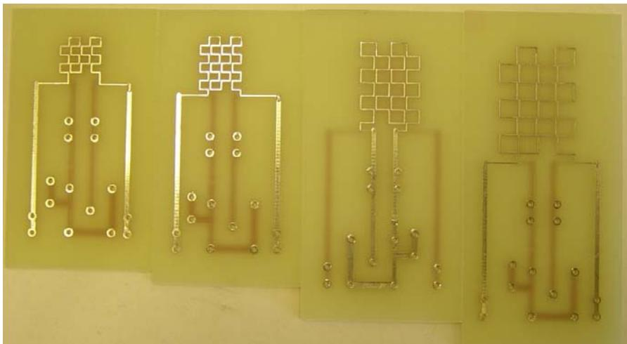
**Figure 5:** Fabricated mesh type sensors, four sizes
