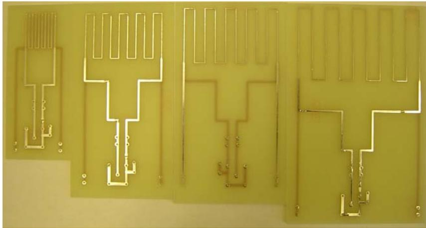
**Figure 4:** Fabricated meander type sensors, four sizes
