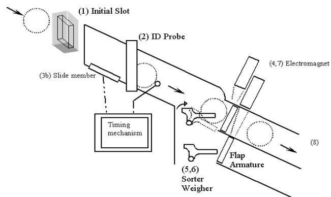
**Figure 7:** Coin Testing Apparatus Schematic
