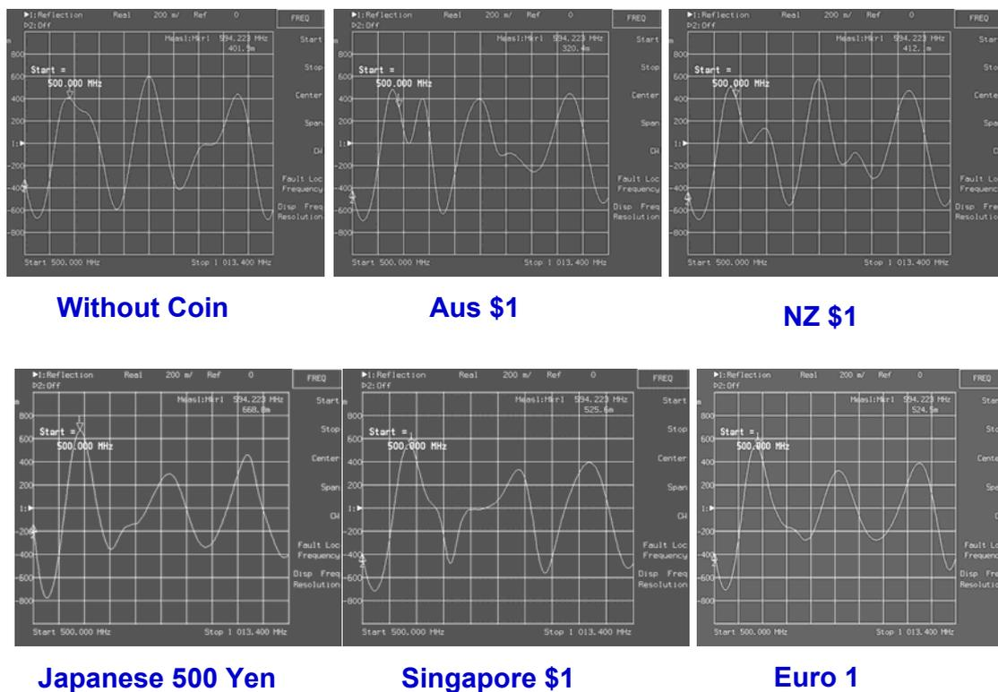
**Figure 15:** Network Analyzer response for different types of coins
